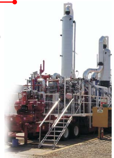
Reclaimer for KMG Red Hawk in the Gulf of Mexico. The first floating cell-spar design
